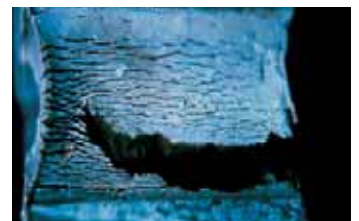
Conventional sealant after 3-month ozone exposure
